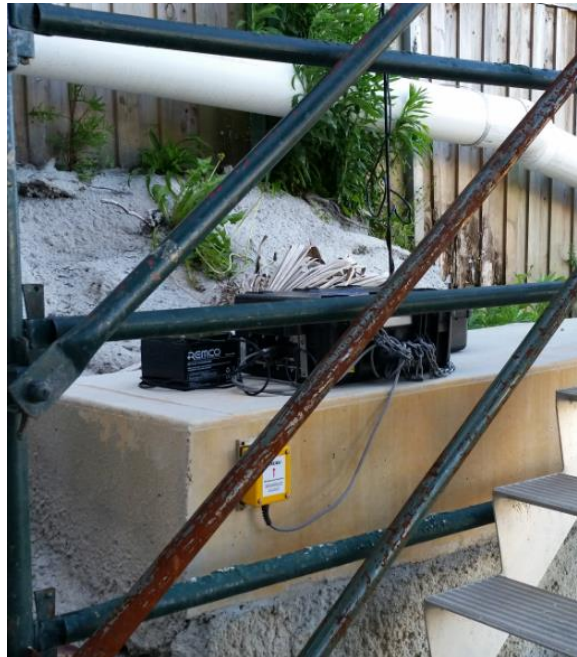
Figure 1 – Vibration Monitor Placement at R1
